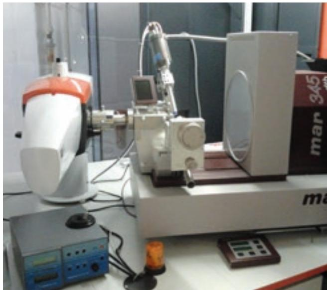
X-ray diffractometer at the Structural Biology Unit.
